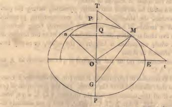
591. Draw M G perpendicular to the ellipse at M, and with the radius O P describe the arc P n.
